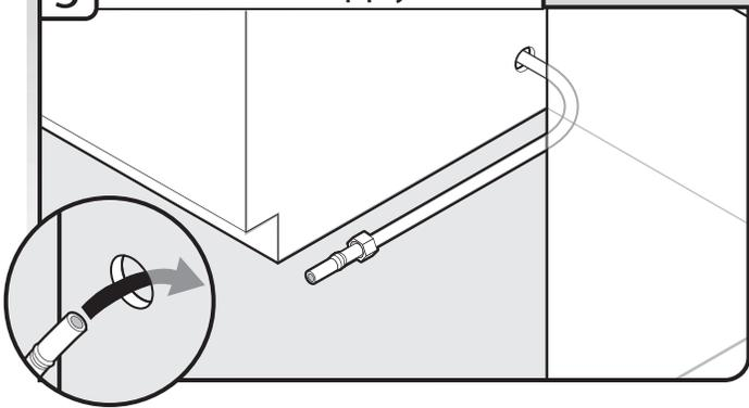
Slowly route water supply line through hole in cabinet. (If using copper tubing, it will bend and kink easily, so be gentle.) It should be far enough into the cabinet opening to connect it to the dishwasher inlet on the front left side of the dishwasher.
